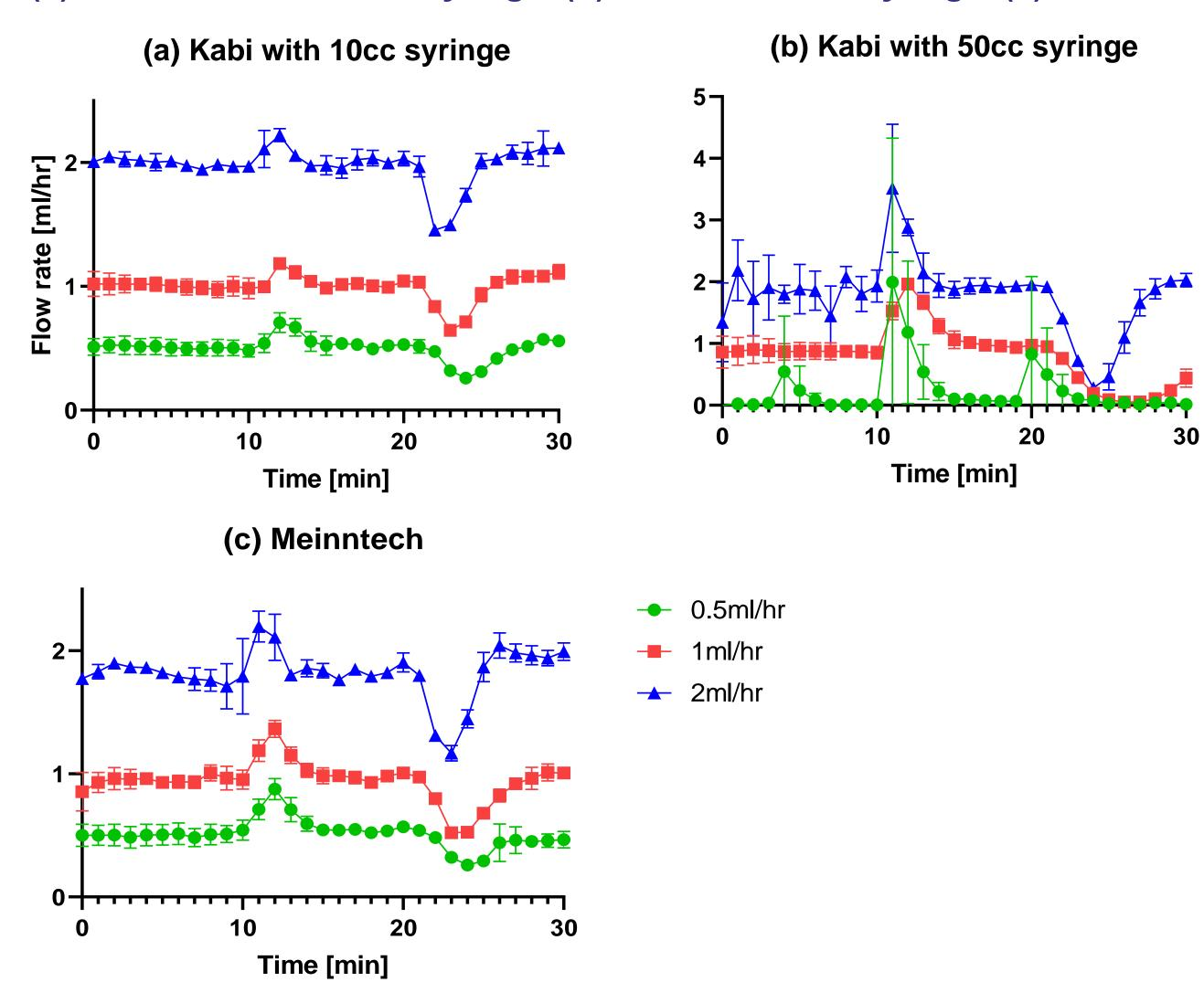
The Kabi pump with 10cc-syringe and Meinntech cylinder pump showed comparable results with IB and ZDDT. However, in case of using a 50cc-syringe in the Kabi pump, significant under-infusion in the slow-rate setting (< 1ml/hr), relatively large IBs and ZDDTs were observed.
