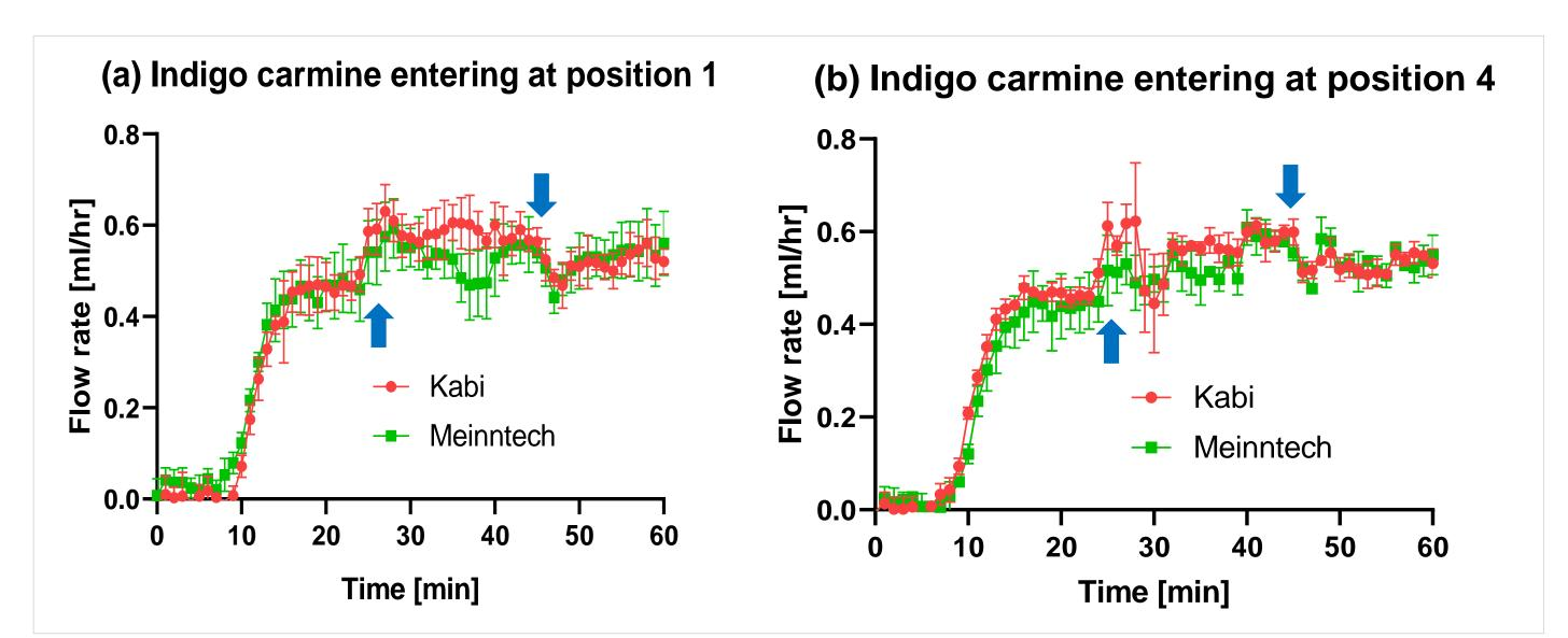
In the multi-infusion setups, starting and stopping the second drug infusion caused an unintentional, transient over-dosing and under-dosing in the first drug delivery, respectively. However, in case of the cylinder pump, its own cartridge acted as an anti-reflux valve to prevent free-flow and siphoning phenomenon.
